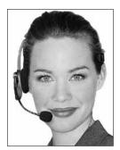
Position microphone near corner of your mouth. Correct positioning ensures that the noise cancellation technology works properly. Slight adjustment of the microphone may help to achieve optimum performance.
