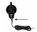
Select charger cord and plug it into the charger port on the headset. Charge for 12 full hours before first use.
